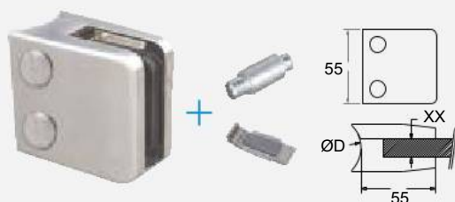
Big Square (55 x 55 mm) with Bottom Plate for Glass 6 to 12.76 mm
